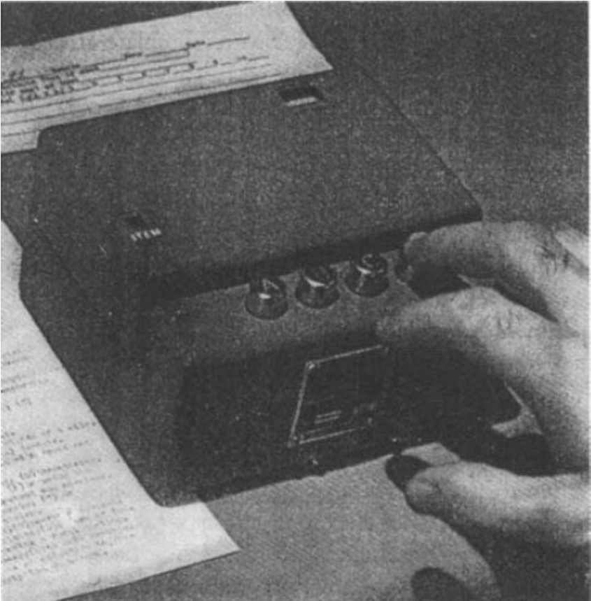
FIG. 1. Pressey's self-testing machine. The device directs the student to a particular item in a multiple-choice test. The student presses the key corresponding to his choice of answer. If correct, the device advances to the next item. Errors are totaled.
