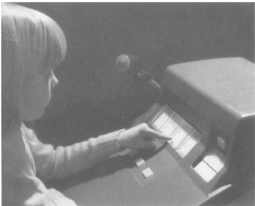
FIGURE 13. A more recent model of a machine to teach matching or related patterns. The machine presents auditory patterns as well as visual. Correct responses move new material into place. The machine can be used to teach both auditory and visual aspects of verbal behavior, music, and so on. It also teaches in the manner of the machines shown in Figures 4 and 5 , a strip of paper being exposed at the right.
