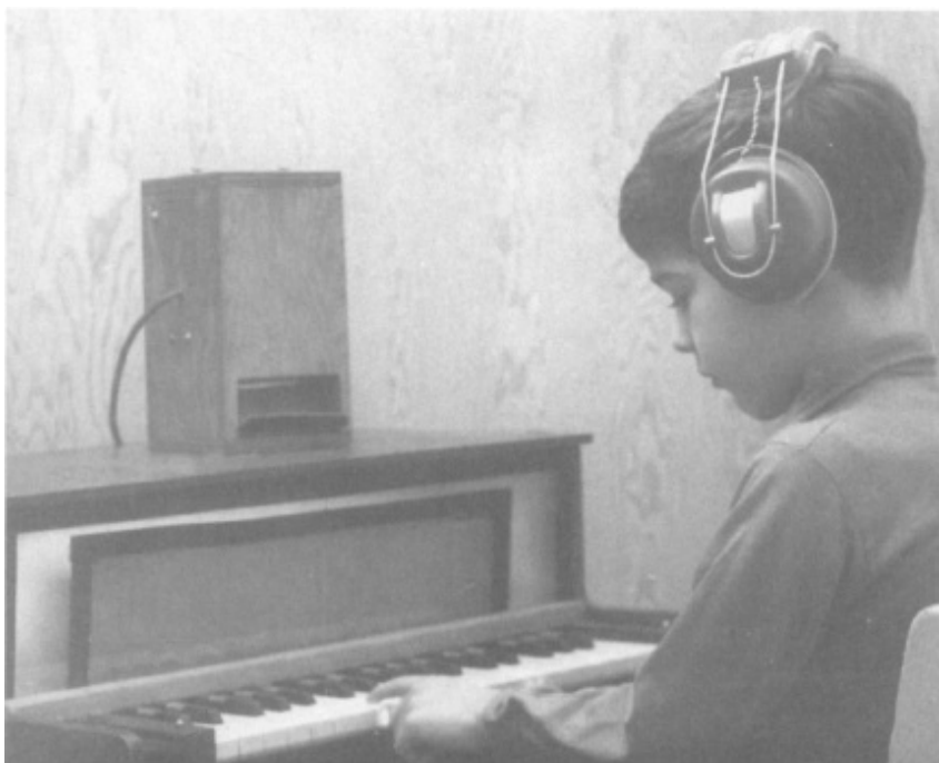
FIGURE 11. A machine to teach “musical thinking.” The machine plays single notes, intervals, melodies, and so on. Keys may be lighted to indicate a set from which matching choices are to be made. Incorrect keys are silent. Correct matches may be reinforced additionally through the operation of the dispenser on the top of the machine which delivers tokens, candies, or coins.
