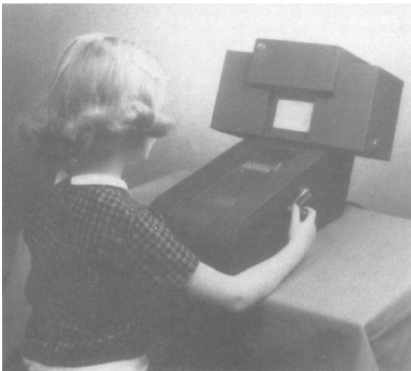
FIGURE 2. A machine to teach spelling and arithmetic similar to that in Figure 1 except that there are more sliders and letters can be presented as well as figures. Material appears in the rectangular opening with one or more figures or letters missing. When the sliders have been moved to complete the material, the pupil turns a crank as shown. If the setting is correct, a new frame of material moves into place and the sliders return to their home position. If the material is wrong, the sliders return but the frame remains and another setting must be made.
