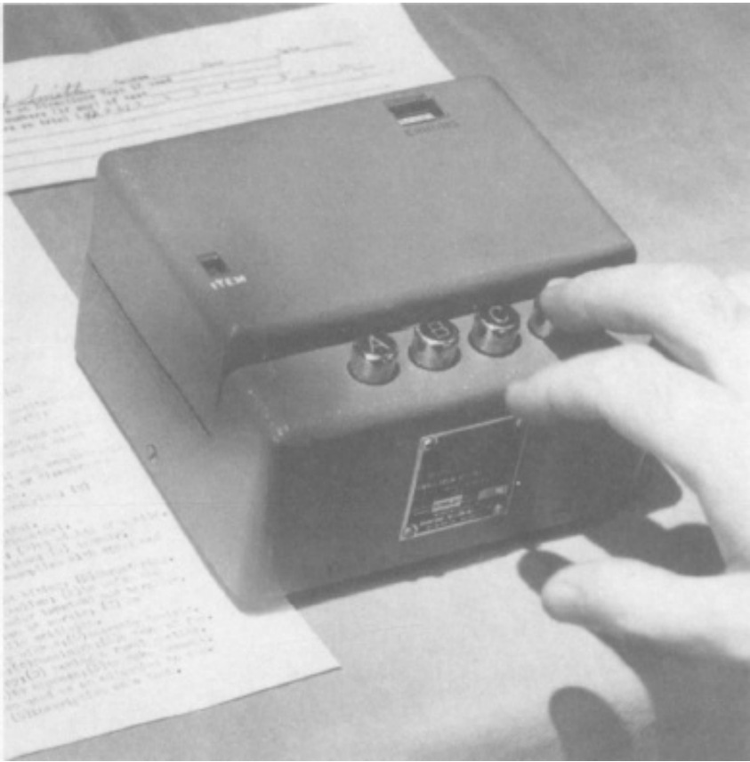
FIGURE 3. A recent model of Pressey's "apparatus which gives tests and scores—and teaches." A number appearing in the window marked "item" directs the student to an item in a multiple-choice test. The student presses the key corresponding to his choice of answer. When he presses the correct key, the device advances to the next item. Errors are totaled.
